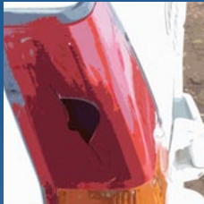
A crack or hole in lamp glass
