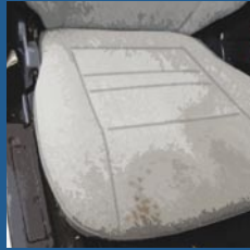
Staining which has damaged fabric texture
