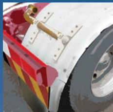
Damaged wheel guards
